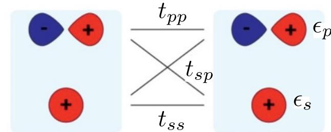
$$H(k) = \begin{pmatrix} \epsilon_s + 2t_{ss} \cos k & -i2t_{sp} \sin k \\ i2t_{sp} \sin k & \epsilon_p + 2t_{pp} \cos k \end{pmatrix}$$
