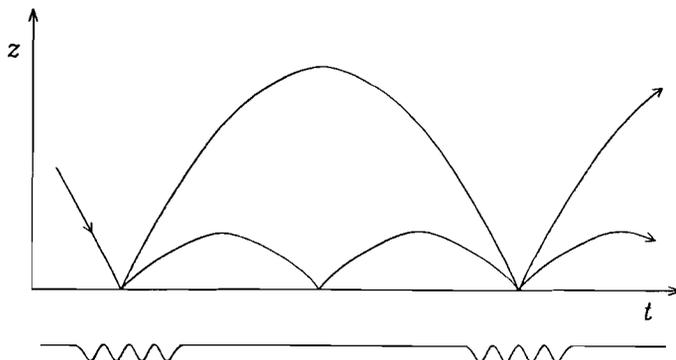
Fig. 6. — Interferometer design in which the interference phase is sensitive to the acceleration due to gravity. Since the vibrating mirror can only transfer a few  $\hbar\kappa$  of momentum, a practical design would involve several bounces before the arms are recombined, as described in the text.
