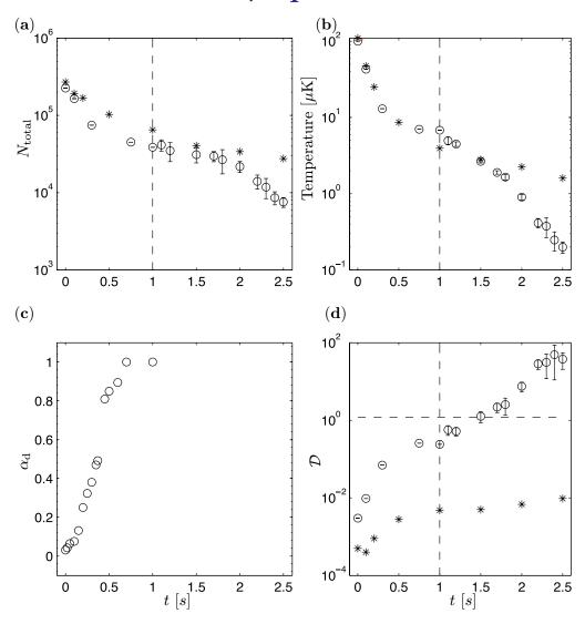
**Figure 5.** Evaporative cooling trajectories in the combined trap (CDT and dT) (circles) and in the CDT alone (stars). We show the time evolution of the atom number N (a), temperature T (b), dimple filling  $\alpha_d$  (c) and phase-space density  $\mathcal{D}$  (d).
